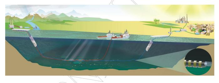
In many places in the world, coastal regions suffer from a shortage of water. However, rivers in other regions pour large quantities of fresh water into the sea. The idea is to take water at the mouth of these rivers. The water removed in this way is transported via a submarine pipe. On arrival, homes, agriculture and industry benefit from the water delivered. This gives rise to a strong economic and social development in these coastal regions.
